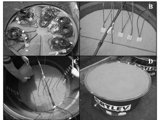
Figure 3. Organization of the TDR probes (A); installation of the probes in the experiment (B), adding soil (C); complete assembly of the experiment (D).
