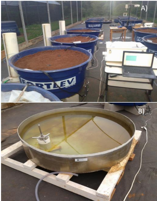
Figure 1. Experimental setup to measure surface (0.05 m) dielectric permittivity ( K_a ) using TDR, lysimeter and auxiliary column used to monitor the water level inside the lysimeters (A); Class A pan used to measure atmospheric demand (B)
